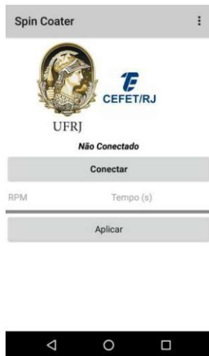
Fig. 2. Image of the Android app created for the user interface. The speed (in RPM) and the rotation time are inserted by the user in the app. The wireless communication is performed via Bluetooth protocol.
