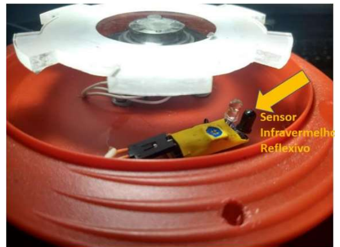
Fig. 3. Final assembly of the first version of the spin coater. The yellow arrow highlights the position where the reflective infrared sensor was attached.
